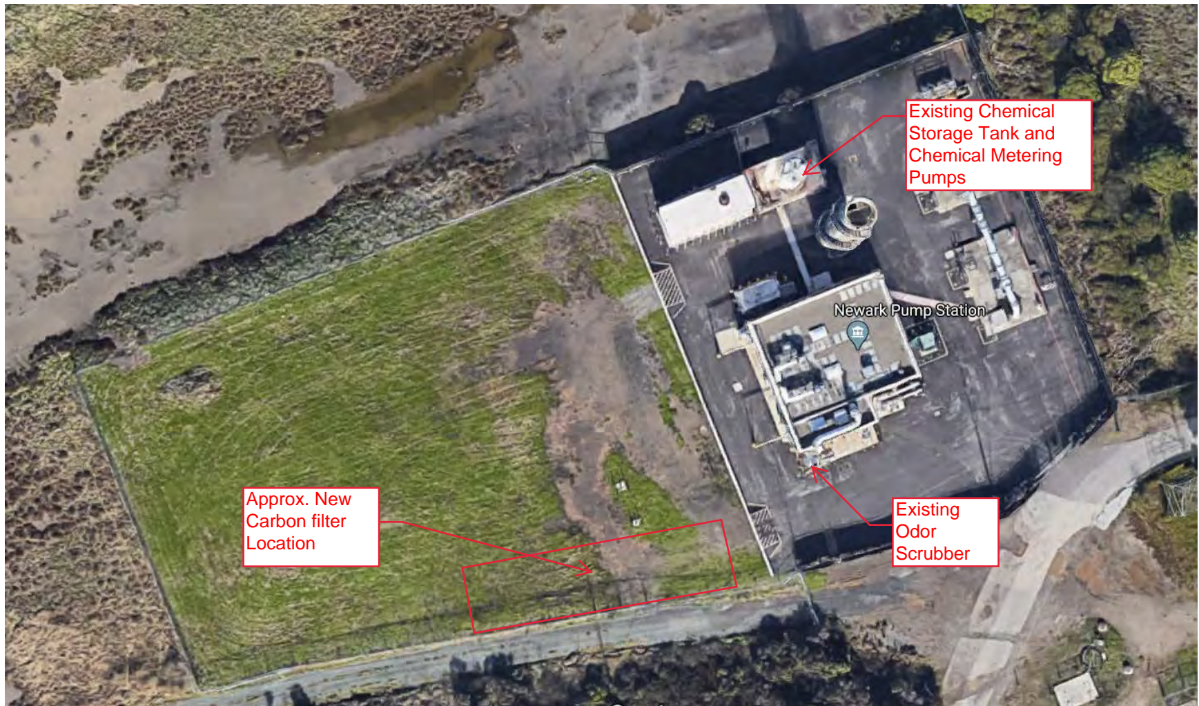
Figure 1 - Newark Pump Station Site Plan
