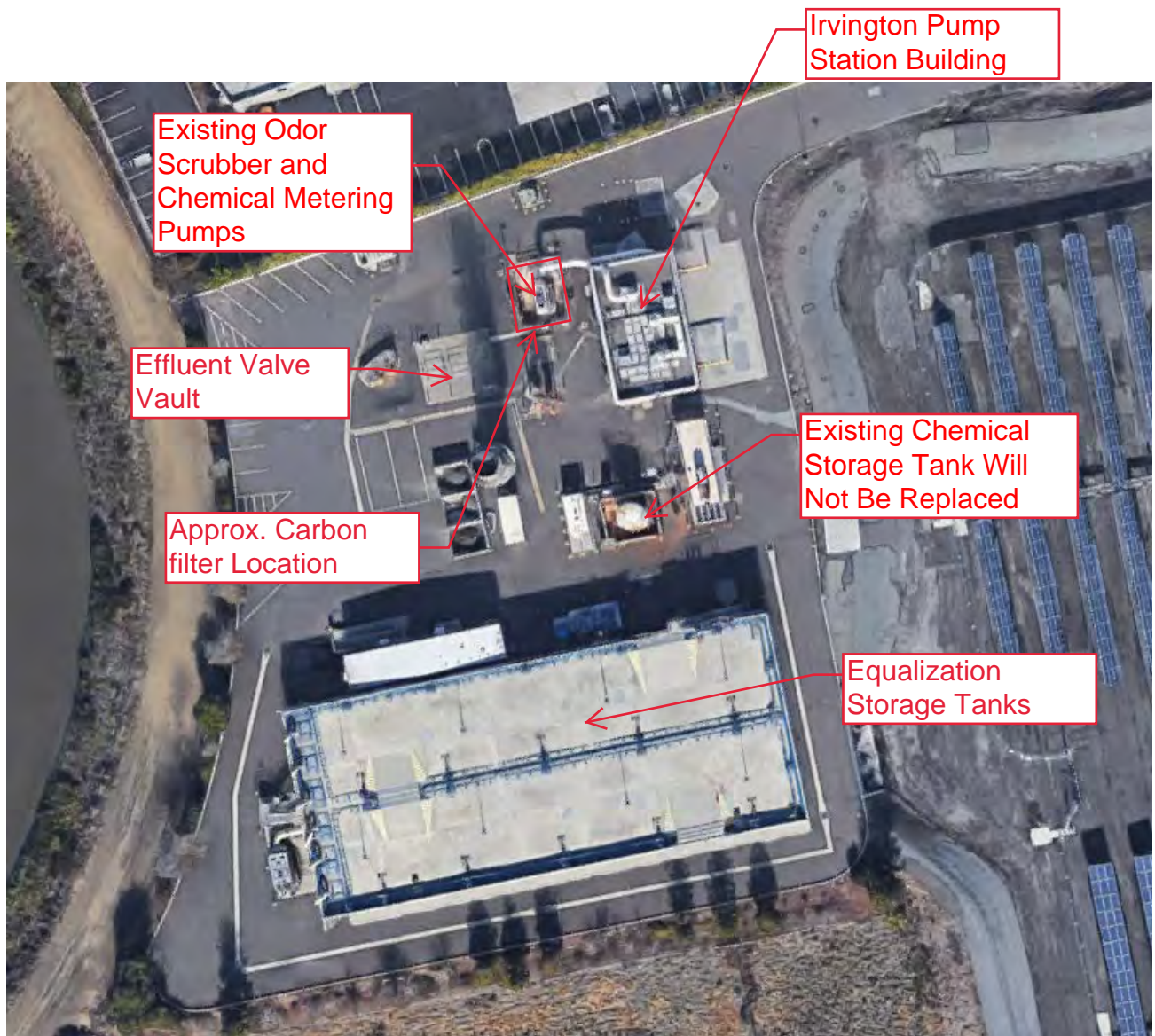
Figure 2 - Irvington Pump Station Site Plan
