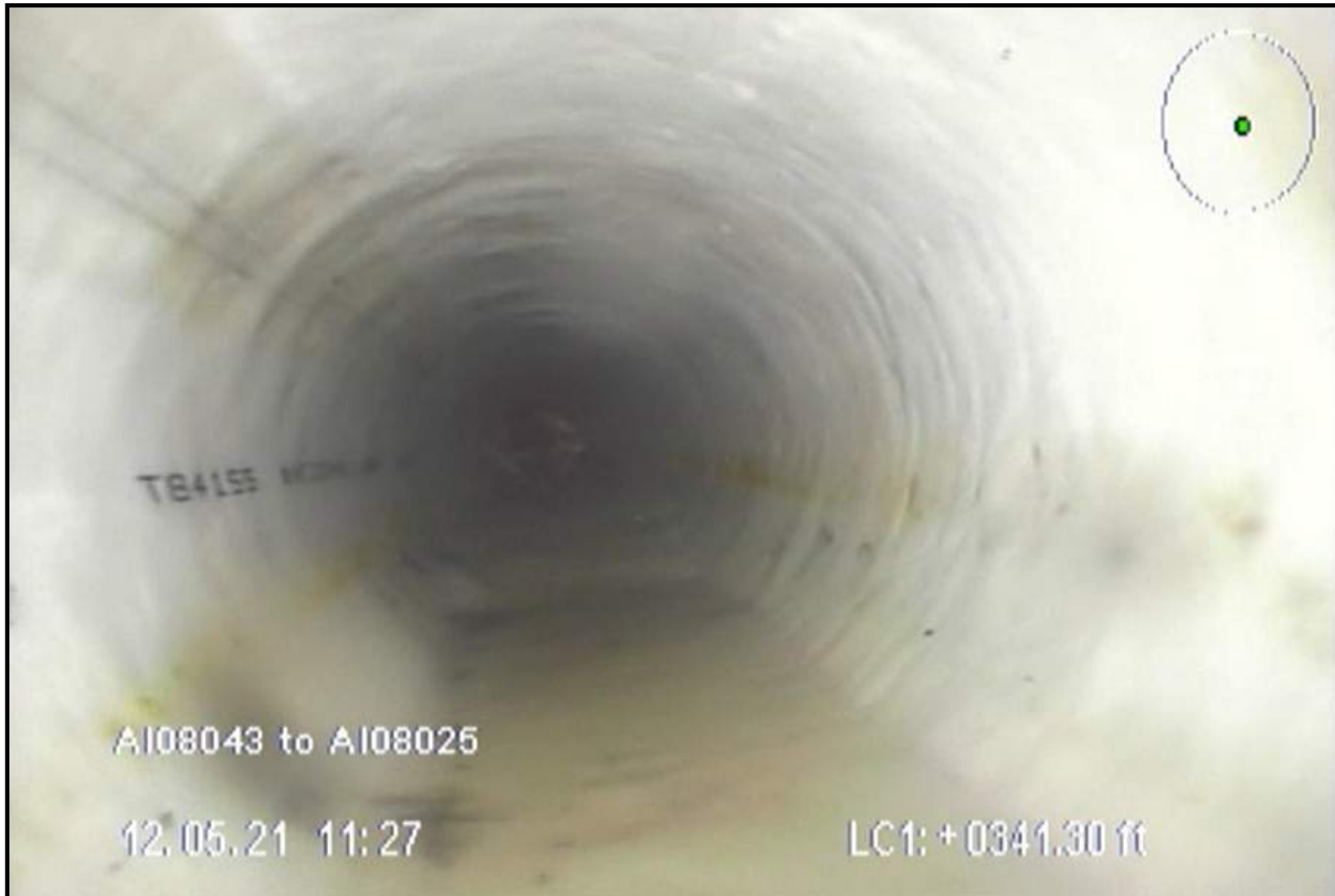
Figure 3 - Site No. 4B, Brier Street, Union City; CIPP Liner Installed.
